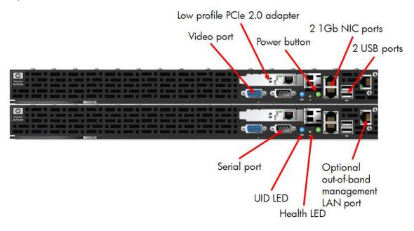
**Figure 4**. Front view of a ProLiant z6000 G6 chassis fully populated with two HP ProLiant SL160z G6 server trays
